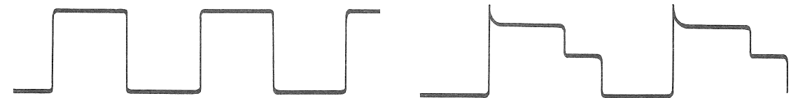
Fig. 2. (A) Waveform present at the cathode of the plug-in multivibrator when the Type TU2 is operating in the Alternate mode. (B) Waveform present at the cathode of the plug-in multivibrator when the plug-in is operating in the Chopped mode.
